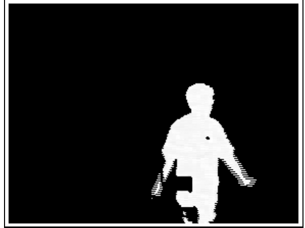
Figure 4: The difference image which provides image forces for the active deformable model.
